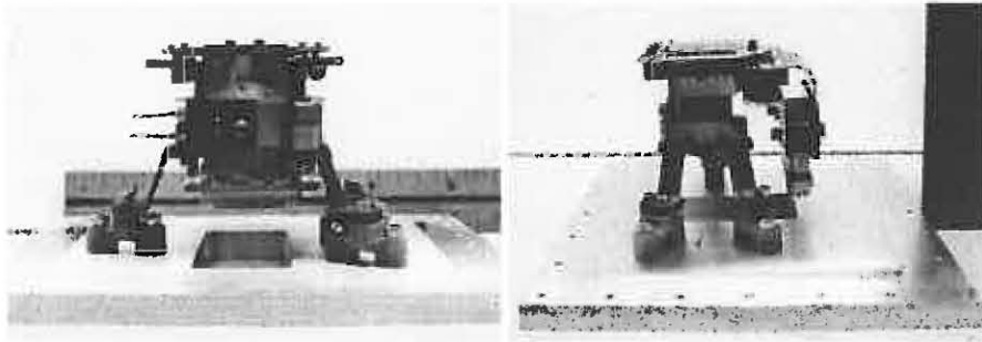
Figure 6. Left: Front view of detector with flight mount prior to vibration testing with launch loads. The (black) heater element of the thermal control system is mounted on a molybdenum block. Not mounted at the time of this picture are the thermal control diode and the thermal monitor diode. These two thermal diodes are located on the molybdenum face opposite the heater and on the molybdenum arm just above the two titanium flexures, respectively. The titanium flexures are mounted on G10-cryogenic standoffs that provide thermal isolation between the 140K detector temperature and the detector housing. The detector cold finger attaches to the copper block below the heater. Right: Side view of detector with flight mount. Note: the bolts were staked prior to vibration testing.
