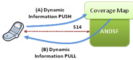
Fig. 3. Dynamic Discovery Procedures: (A) PUSH of information from the UE to the Coverage Map, (B) PULL of information to the UE through the ANDSF decisions
