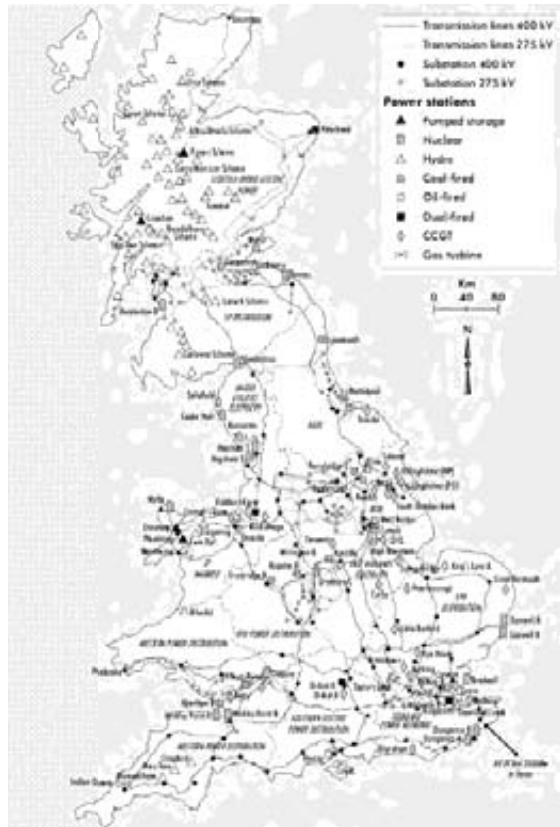
Figure 8.2: Great Britain’s Transmission Network 48
