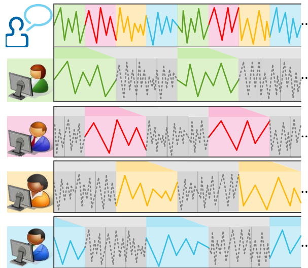
Fig. 14. TimeWarp forwards different “warped” versions of the audio to each worker. Workers hear a slowed down version of the content they are supposed to caption, while they hear the rest sped up. This increases the quality of workers’ output by asking them to complete an easier task without losing context. The start of each segment is aligned with the original audio, allowing the crowd to collectively caption in real-time.
