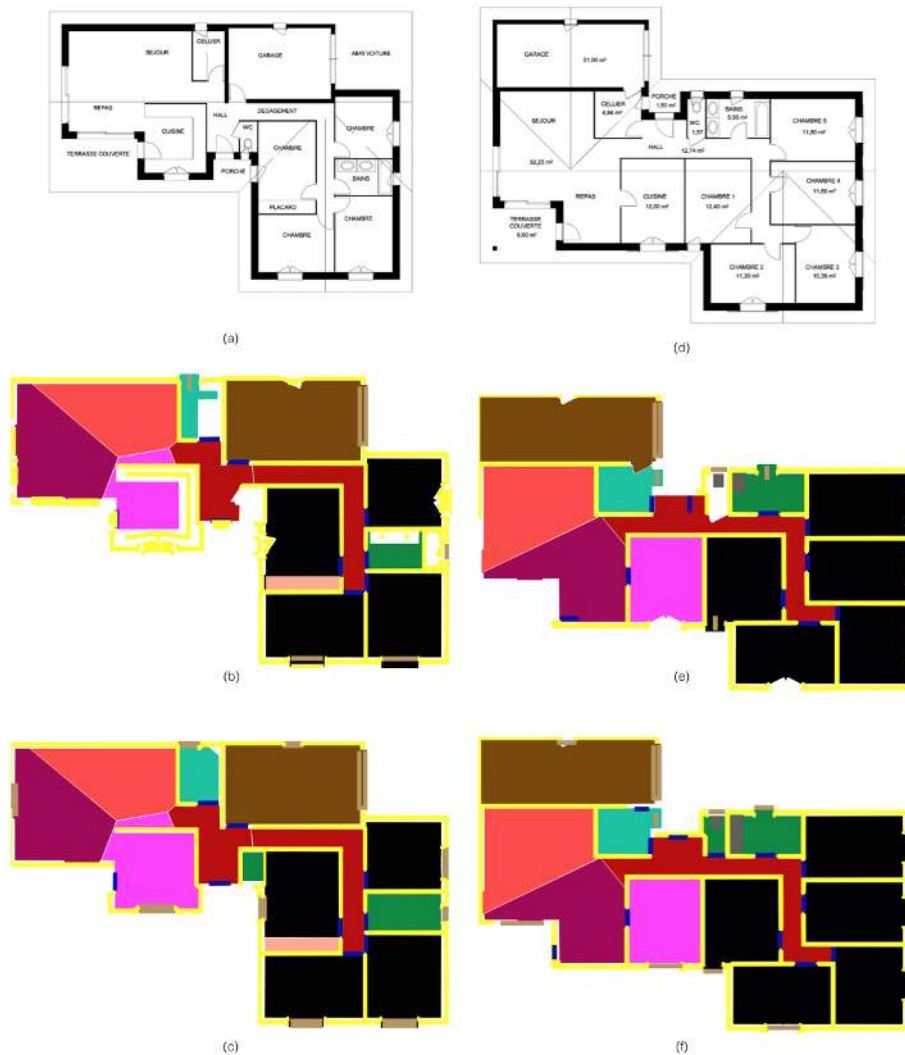
Figure 6: Test graphics: Input images (a, d), uncorrected graphics (b, e), and corrected graphics (c, f).
