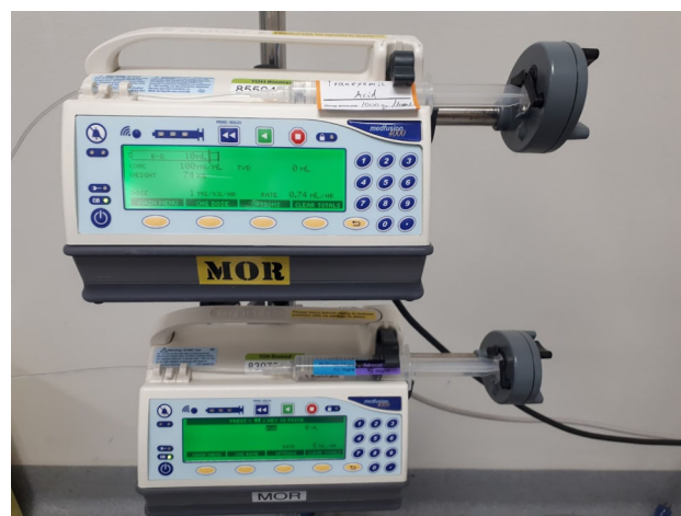
Fig. 2 Replicated set-up of syringe infusion pumps with tranexamic acid in a 10-mL syringe (top) and epidural solution in a 20-mL syringe (bottom).
