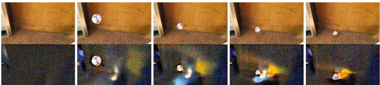
Fig. 13 Relaxing the anti-pinhole camera. This figure shows some frames of a video showing a ball bouncing and the difference between a frame without ball present and the frames of the video. The difference
