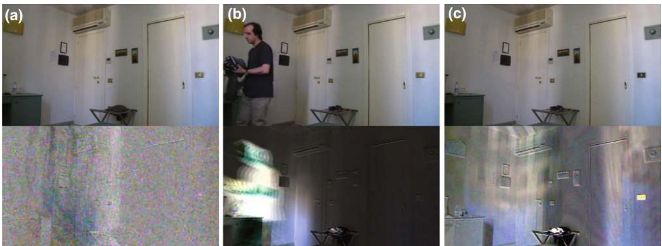
Fig. 16 Three frames from a video of a person walking inside a room. Top row shows the three unprocessed frames, and the bottom row shows the difference of multi-frame average centered on current frame from a multi-frame average of the background. (a) One of the first frames in the video. (b) A person inside the room blocks some of the light
