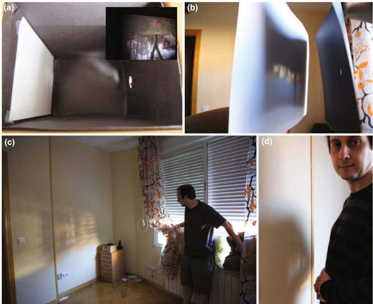
Fig. 3 Relaxing the pinhole camera design. (a) Pinhole camera from a class project (the small thumbnail shows a picture taken with this camera). (b) Relaxing the design of the pinhole camera by removing the walls of the camera. (c) Turning the room into a camera obscura using
