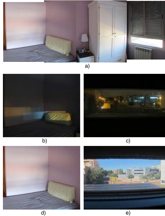
Figure 3. Examples of convolutions by the aperture function. (a) Lighting within room shown together with the window opening. (b) Lighting from a night scene, and (c) the view out the window at night, showing the multiple point sources. The point sources reveal in (b) the rectangular convolution kernel of the window aperture. (d) Daytime view within the room, and (e) the view out the window, which, convolved with the window aperture, yields the projected patterns in (d).
