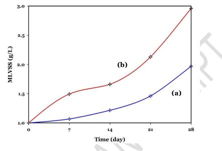
**Fig. 5.** The changes in MLVSS of the reactor without biochar supplementation (a), and with biochar supplementation (b).
