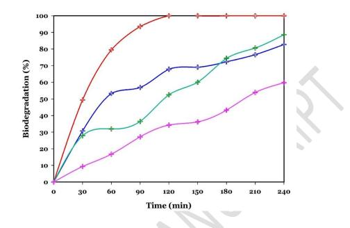
Fig. 7. Phenol biodegradation potential of the acclimatized sludge (%) under different initial phenol concentration, MLVSS values have been presented in Fig. 5. —↑— 25 mg/L, →— 50 mg/L, →— 100 mg/L, →— 250 mg/L
