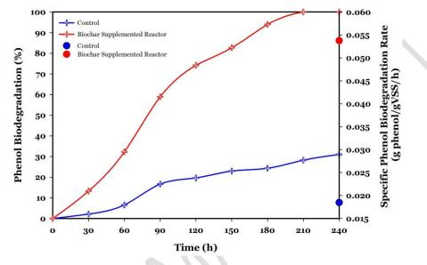
**Fig. 12.** The performance of the anaerobic sludge acclimatized in presence of pinewood biochar compared to control (without biochar supplementation) under initial phenol concentration shock (to 500 mg/L).
