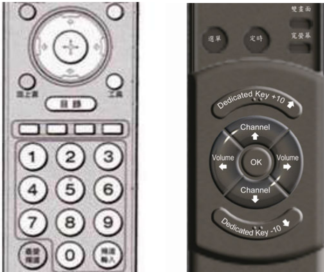
Fig. 2. The design of multi-layer TV remote controller was developed that hiding less frequently used buttons and rearrange frequently used buttons on the easily reachable surface of the TV remote controller
