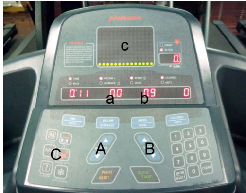
Fig. 1. The function keys are marked A, B and C; while their corresponding display screens are marked a, b and c respectively. (A: incline, B: speed, C: six types of program)
