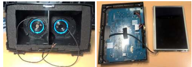
Fig. 3. Overview of the HMD design. (Left) Optotune lenses and the 3D printed holders. (Right) Detachable screen.
