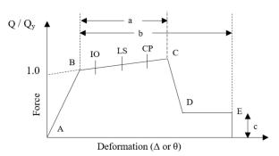
Figure 9. Generalised force deformation curve as per ASCE 41–17 [54].
