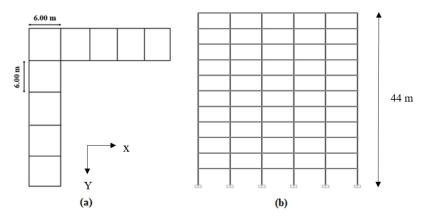
Figure 1. Geometric orientation of unsymmetrical building: (a) plan view; (b) elevation.
