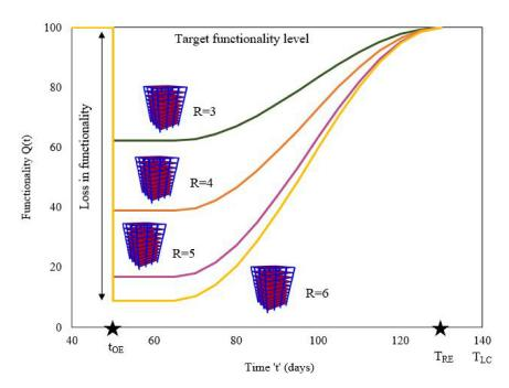
**Figure 8.** Graphical representation on functionality curves with respect to R factor. The time of occurrence of a seismic event is designated as  $t_{OE}$ , its recovery time is designated as  $T_{RE}$ .
