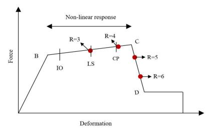
**Figure 11.** Schematic representation of variation in the building performance level with respect to R factors at the MCE design level under bidirectional loading.
