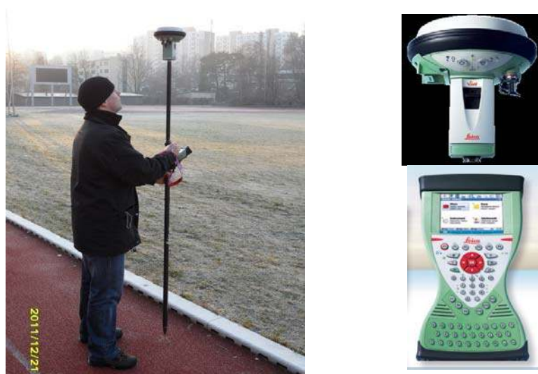
Fig. 8. Taking inventory measurements of the stadium and GNSS receiver with a controller [own study]
