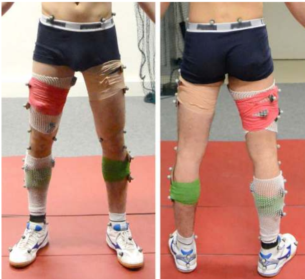
Figure 1. Subject equipped with 30 reflective markers (14 single markers and 16 markers on technical clusters placed on both thighs and shanks). A technical marker was placed on the left iliac crest only for labelling purpose. Foot markers were not included in this study. Markers were placed by skilled experimenters who received a training in palpatory anatomy.
