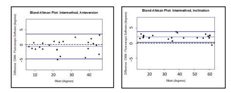
**Figure 7.** Bland–Altman limits of agreement for the intermethod analysis comparing the software analysis to the CMM analysis for the cup only images.
