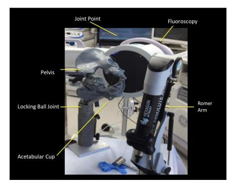
**Figure 1.** Experimental set-up including pelvis model secured with acetabular component in place, fluoroscopy unit, and the coordinate measure machine Romer Arm.
