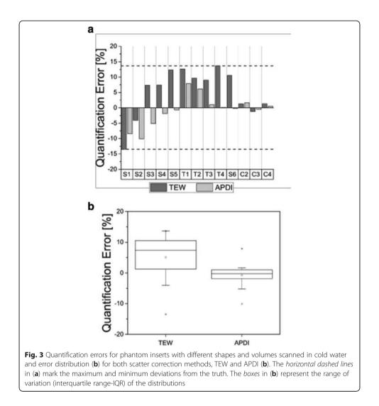
in each object. Therefore, in general, the accuracy of activity quantification achieved in these experiments was very good; activities reconstructed with TEW scatter correction differed for most of the objects by less than 5% from the true values. These results confirmed that our reconstruction method perform well in low scatter and attenuation conditions.
