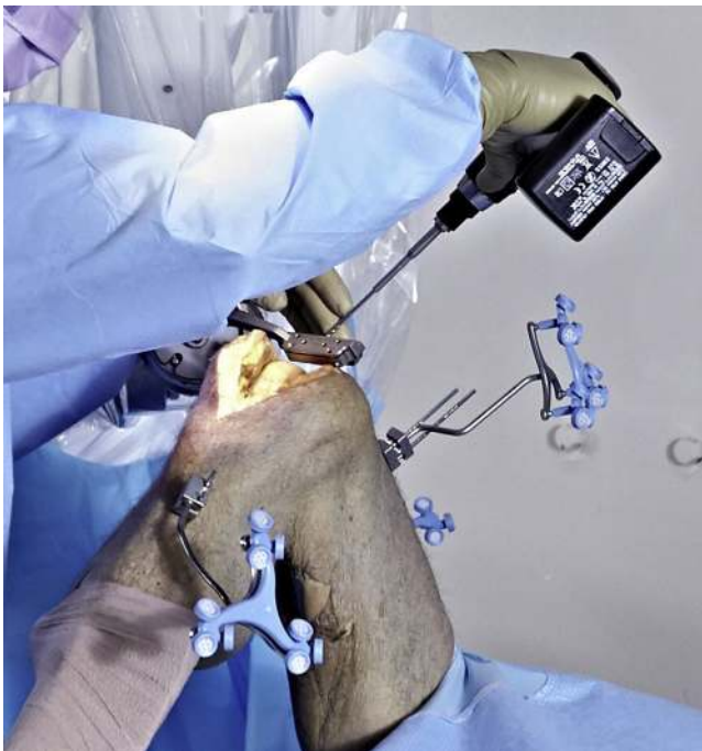
Fig. 2. The principle of ROSA Knee surgery is simple: the Robotic arm positions and holds the universal cutting jig in the desired location as determined by the surgical plan. Once the cutting jig is set in the correct position it is pinned to the bone and the surgeon then performs the cuts.
