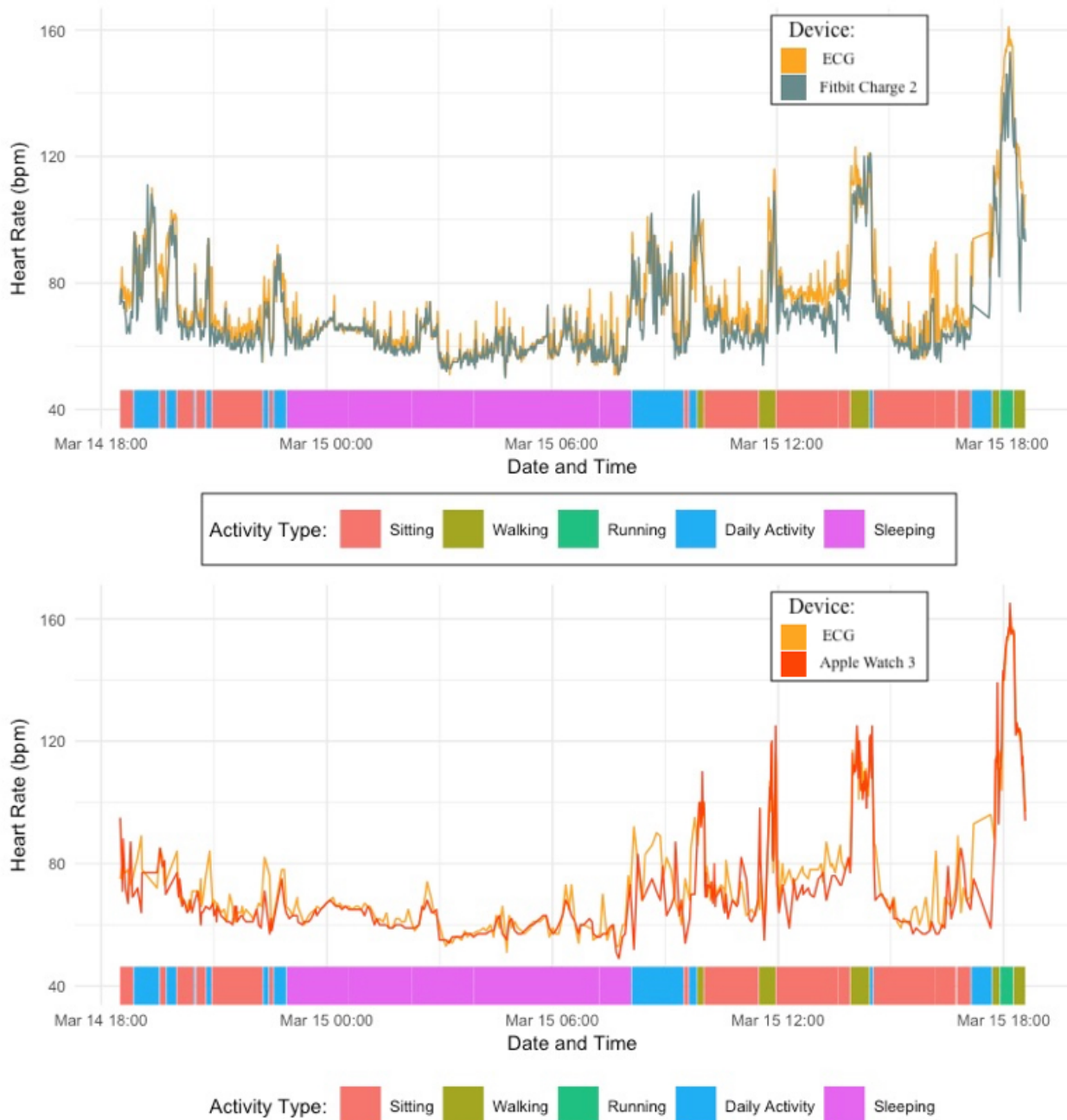
Figure 2. Fitbit Charge 2 (top) and Apple Watch 3 (bottom) compared to the electrocardiogram (ECG) across 24-hours. bpm: beats per minute.
