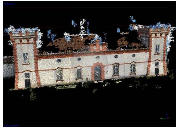
Figure 11. Point cloud obtained from model M3: front façade of the castle.
