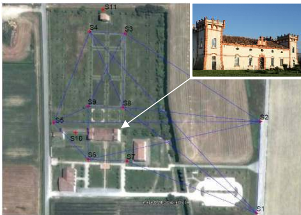
Figure 2. The 3D reference network
