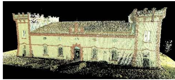
Figure 3. The TLS point cloud model of the Castle
