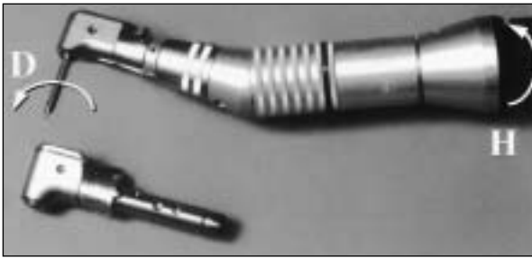
Fig 1a (Top) The Nobel Biocare mechanical torque-limiting device. An assembled 10-Ncm torque wrench with rotating handle (H) and driver (D). (Bottom) A 20-Ncm handpiece head that can be installed in place of the 10-Ncm handpiece head.
