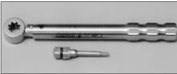
Fig 1c The DynaTorq ITL mechanical torque-limiting device and (top) and a hex driver (bottom).
