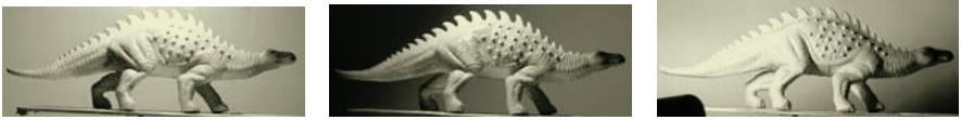
Fig. 5. Three out of 15 images with extremely near light (20 cm) used for photometric stereo reconstruction.
