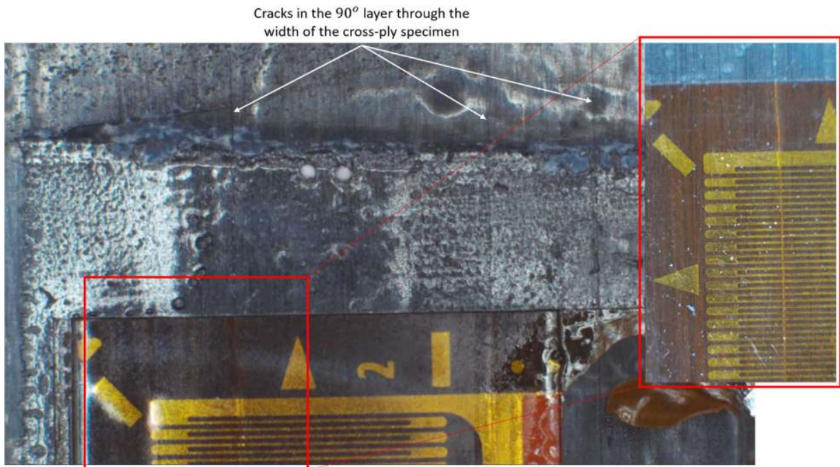
Figure 9. Local failure of the 90^\circ layer for the cross-ply configuration.
