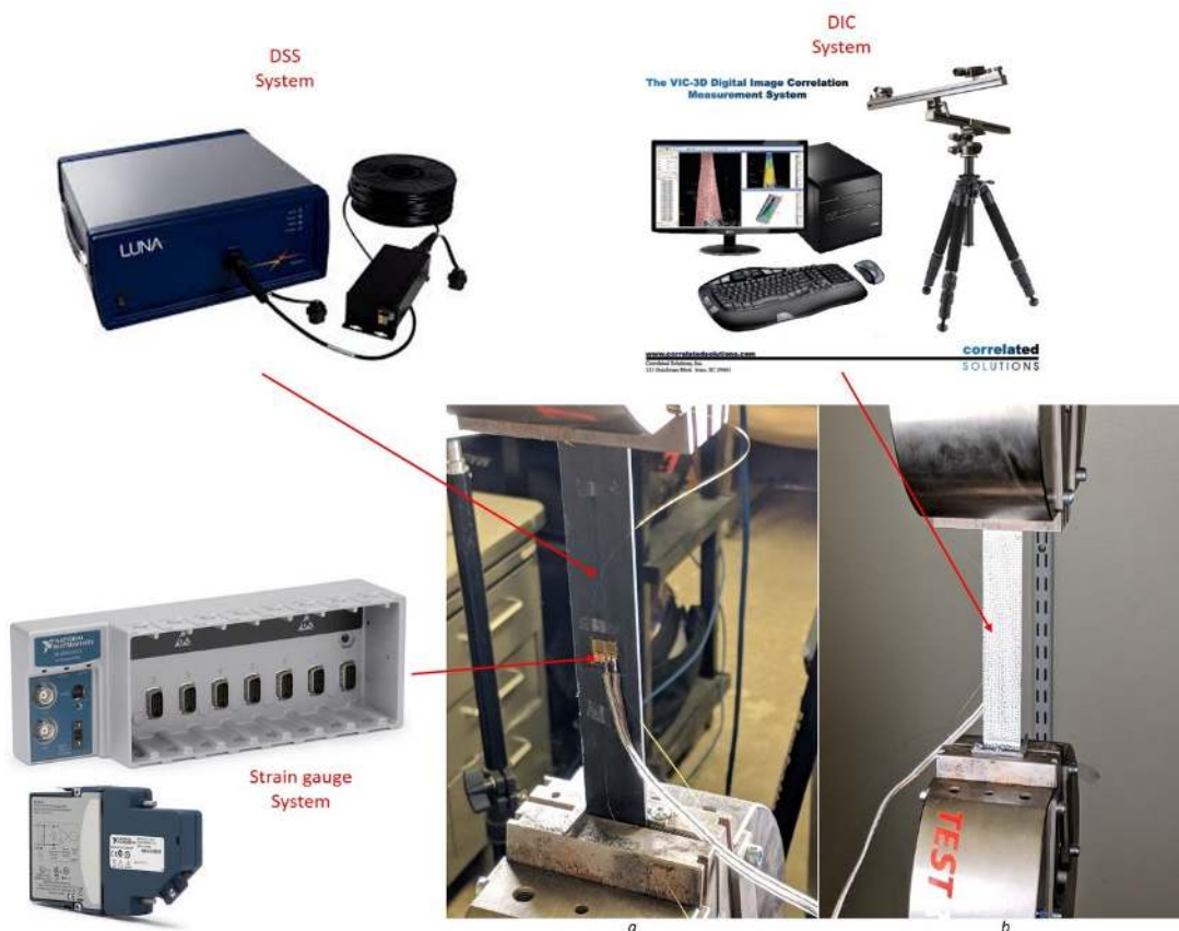
Figure 1. Strain gauges and DSS instrumented on the back surface of the specimen (a), speckle pattern for the DIC system on the front surface of the specimen (b).
