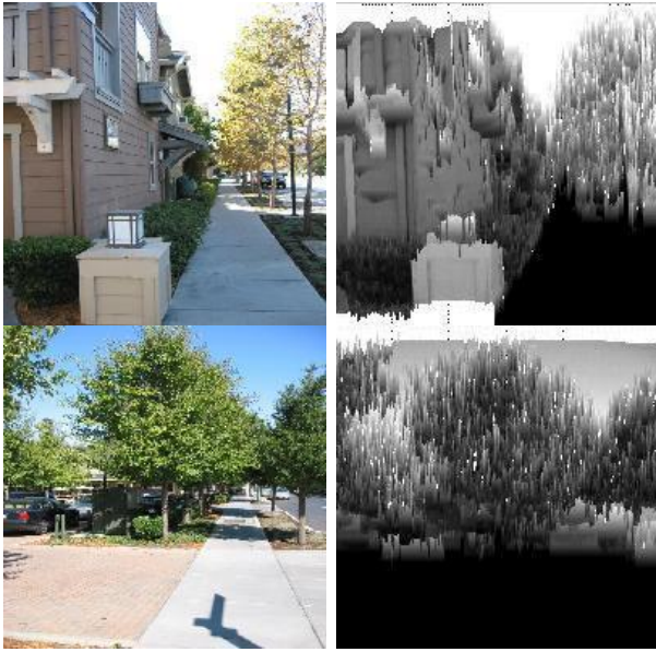
Fig. 12. Left figures show the original images. Right figures show the 3D reconstructions based on the estimated ground plane. The black region in the images on the right shows the estimated ground plane.
