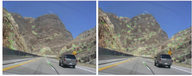
Figure 2. Inlying feature projections obtained using the standard KLT tracker (left), and the guided KLT tracker introduced in this paper (right).
