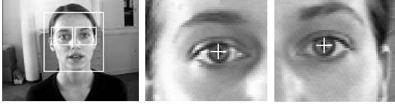
Figure 1: Multi-stage approach for eye centre localisation. A face detector is applied first; based on the face location rough eye regions are extracted (left), which are then used for a precise estimation of each eye centre (middle and right).
