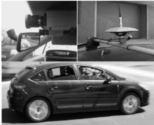
Fig. 6. (Top left) Stereo cameras. (Top right) RTK-GPS. (Bottom) Experimental vehicle.
