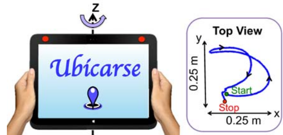
Figure 1: Twisting the Mobile Device. The user twists the device about its vertical ( z ) axis, as shown in the figure on the left. The red circles indicate antenna locations. On the right, we depict the top view of a candidate device trajectory as measured by a Vicon motion capture system.
