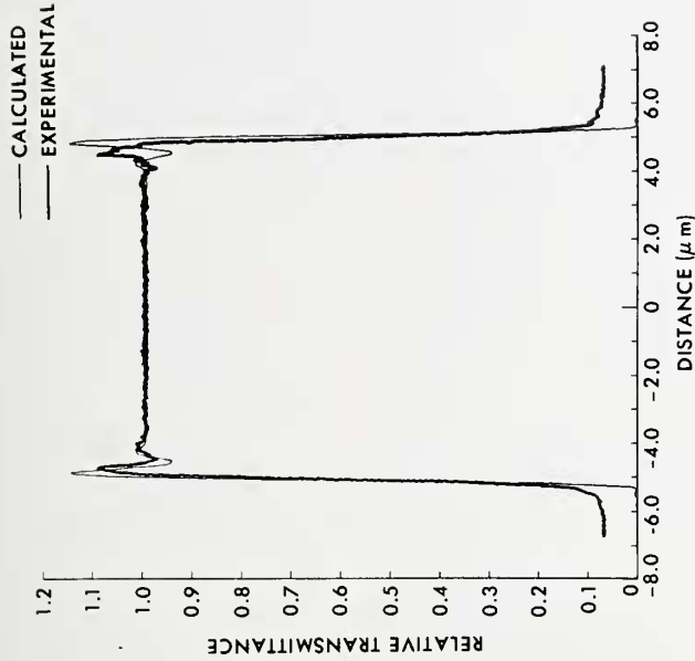
(b) 0.90 N.A. objective and 0.22 N.A. condenser; most coherent case.
