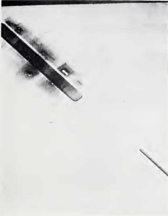
Figure 5-3. SEM photomicrograph showing contamination from repeated scans across a nominally 3- \mu\text{m} wide clear line on an AR-chromium artifact; SEM operating voltage of 10 keV and magnification of 1700X.
