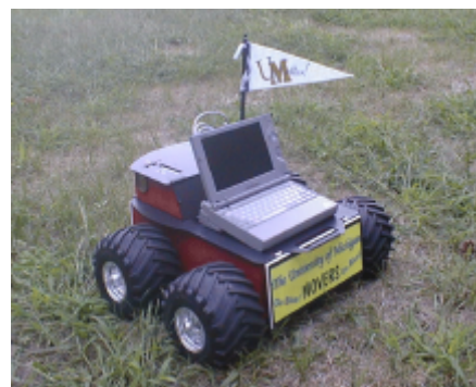
Figure 4: The University of Michigan's Pioneer AT robot used in the experiments described here.
