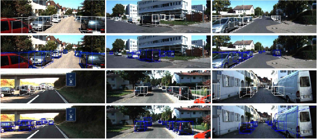
Figure 5. Qualitative comparisons of 3D detection results: 3D Boxes are projected to the image plane. White boxes represent our predictions, and blue boxes come from ground truth.
