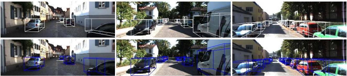
Figure 6. Qualitative comparisons of RGB information: 3D Boxes are projected to the image plane. The detection results using XYZ information only are represented by white boxes, and blue boxes come from the model trained with RGB features fusion module. The proposed RGB fusion method can improve the 3D detection accuracy, especially for occlusion/truncation cases.
