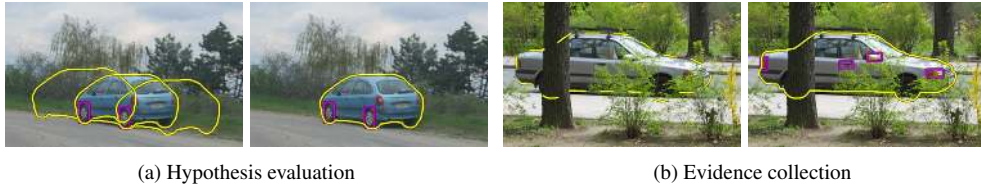
Figure 3. Main points of our framework. (a) Ambiguities introduced by local features may generate false hypotheses (left). Hypothesis evaluation helps to avoid them in our framework (right). (b) Occlusion weakens the discriminative classifier response and the object may be missed (left). This is reduced in our framework by collecting the local evidence provided by agreeing features (right).
