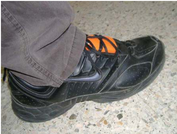
Fig. 1. Xsens IMU attached to the right foot using the shoe's laces.
