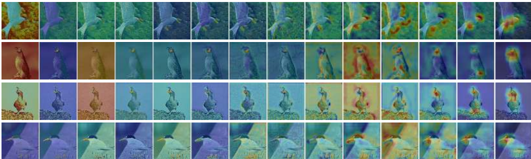
Figure 8: Illustration on extending CAM from the last layer to all layers with ACDC-net . In CAM, the visualized heatmap explains the importance of image regions. Each row shows the class activation maps of a sample from the first convolution layer (left) to the final convolution layer (right).
