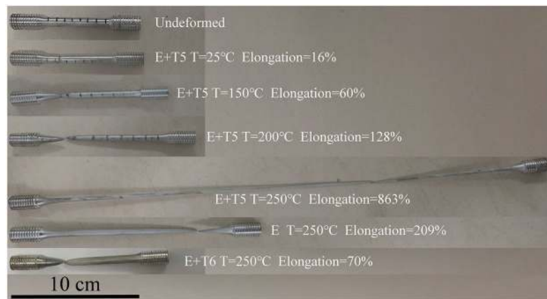
Figure 2. Representative initial and fractured tensile specimens for superplastic deformation of GZ57K alloy.
