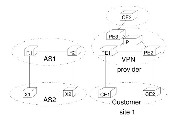
Fig. 3. The parallel-links problem for peering links and BGP/MPLS VPNs
