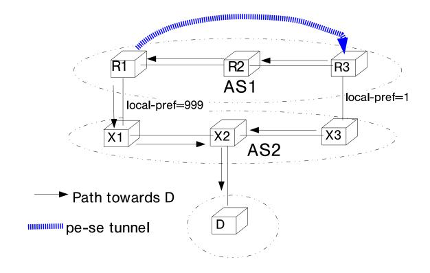
Fig. 10. Example topology for the deactivation of a pe-se tunnel
