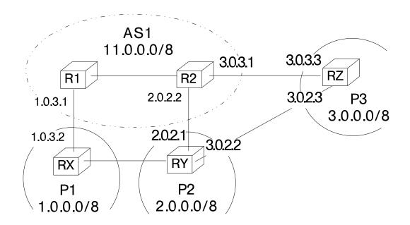
Fig. 9. A stub AS attached to three providers
