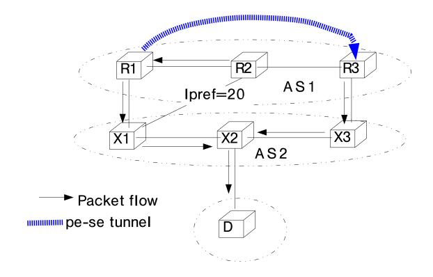
Fig. 8. Utilisation of a *pe-se* protection tunnel
