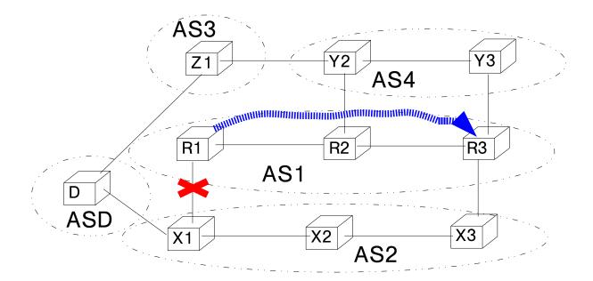
Fig. 11. BGP convergence with a *pe-se* protection tunnel
