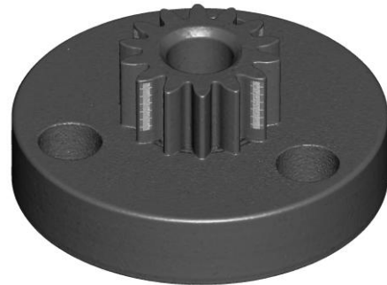
Micro spur-gear with tactile measured flanks and 3 holes on mounting base (2 visible)
