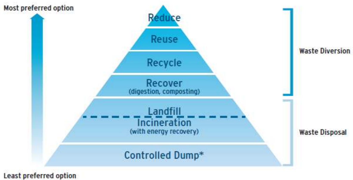
Figure 7. An example of the solid waste hierarchy, describing how integrated solid waste management activities should relate to different treatment methods. The top and thereby most preferable waste treatment options Reduce, Reuse and Recycle (the three R's) does together with Recover forms the options of waste diversion. The least preferred options Landfill, Incineration and Controlled dumping are examples of waste disposal. *Controlled dumping is the very last option to be accepted. Uncontrolled dumping should at all costs be avoided. (The World Bank, 2012)
