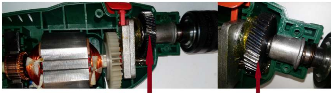
Broken tooth on sprocket
