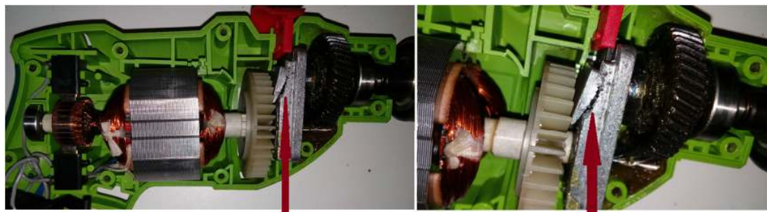
Damaged gear train
