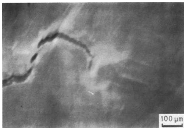
Figure 7 Photograph of sliding between crack surfaces and the potential for friction emission.
