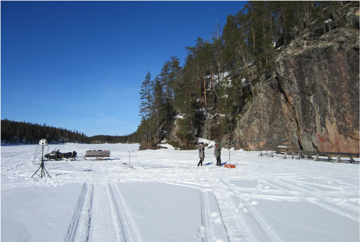
Fig. 3 Recording setup on ice in front of the Värrikallio cliff. From left: the dodecahedron loudspeaker, the snow mobile with a sledge, the recording and playback devices, researchers Tiina Äikäs and Annu Mikkonen, the tetrahedron microphone array, the spectator pier and the painted cliff. Photograph: Riitta Rainio
