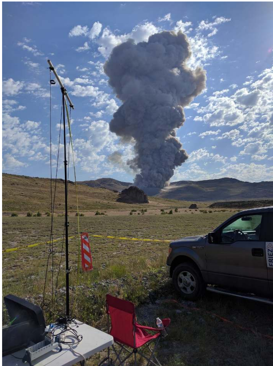
Figure 2. Example of the intensity microphone setup at 120°, with the rocket exhaust pictured in the background.
