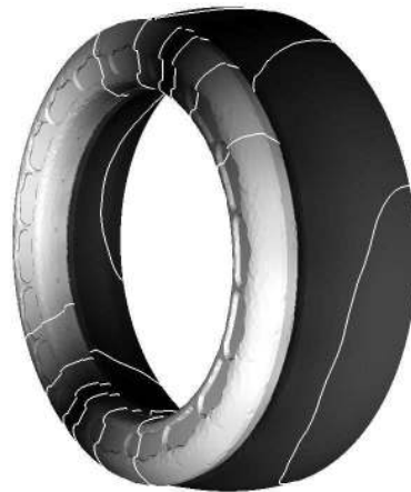
d: First orthoradial/first longitudinal mode - f = 896 Hz
