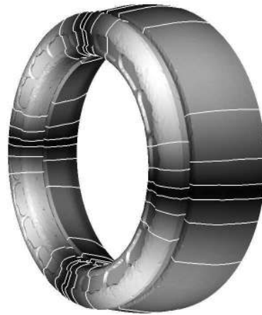
b: Second orthoradial mode - f = 686 Hz
