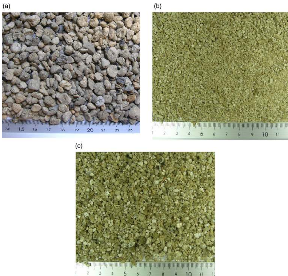
FIGURE 1. Morphology of the three types of lightweight aggregates used: (a) arlite; (b) vermiculite type 2 and (c) vermiculite type 3.
