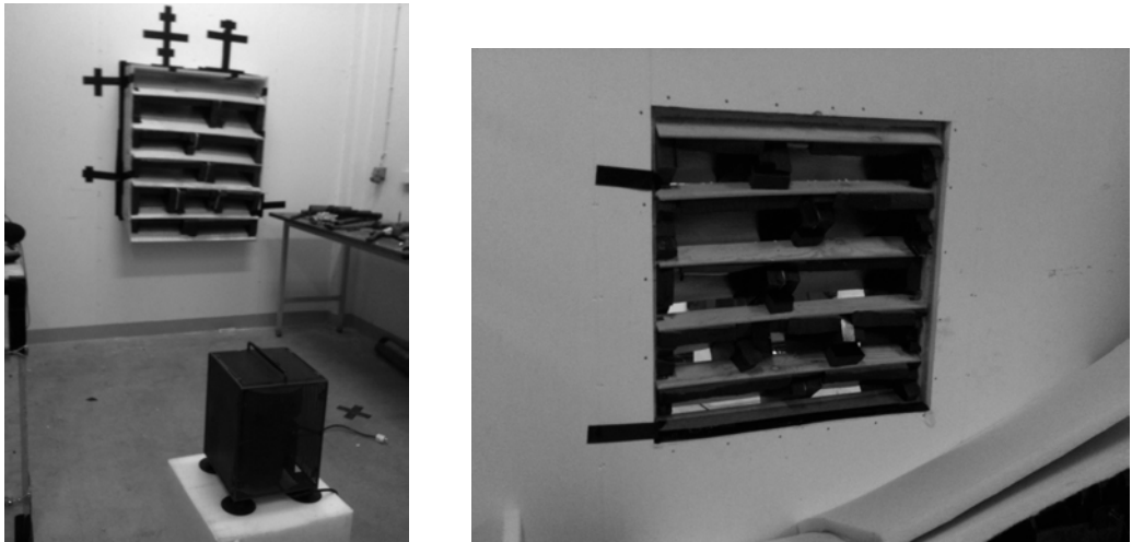
Figure 6.12.: Measurements of the improved baffled panel in the laboratory.
