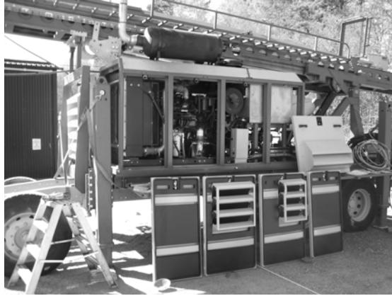
Figure 1.2.: Photo of the power pack without encapsulation.
