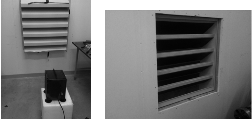
Figure 4.17.: Photos of the setup for the laboratory measurements of the transmission loss of the front baffled panel.
