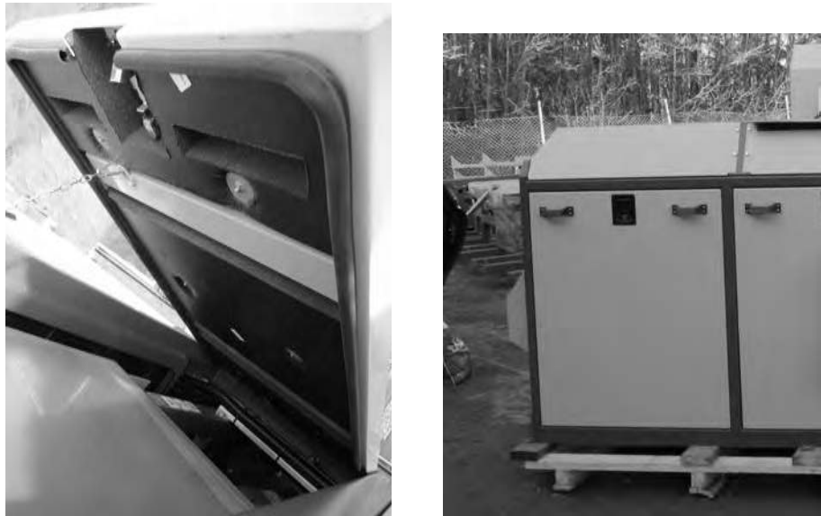
Figure 1.3.: Photos of the solid panel of the encapsulation from inside of the power pack (left) and from outside (right).
