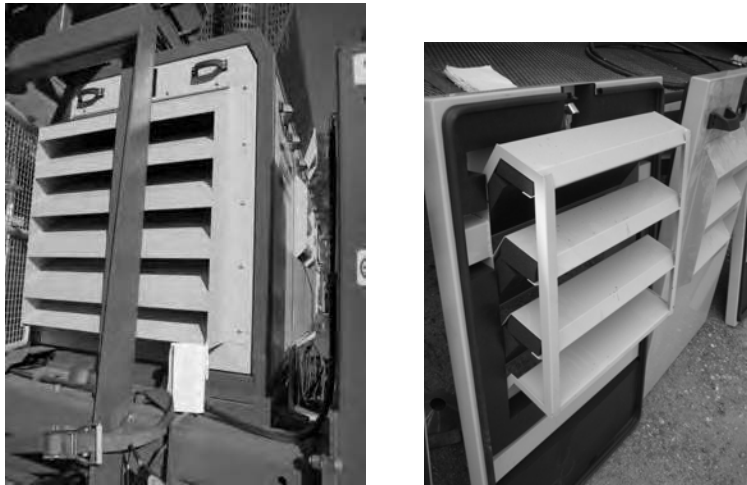
Figure 1.4.: Photos of the front baffled panel (left), the chevron-blade baffled side panel (right)
