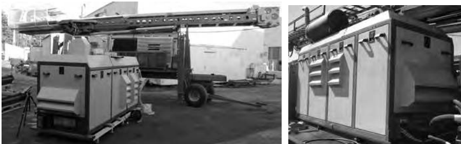
Figure 1.1.: Photos of the power pack's encapsulation in front of the power pack unit (left), and the encapsulated power pack with core drilling rig (right).
