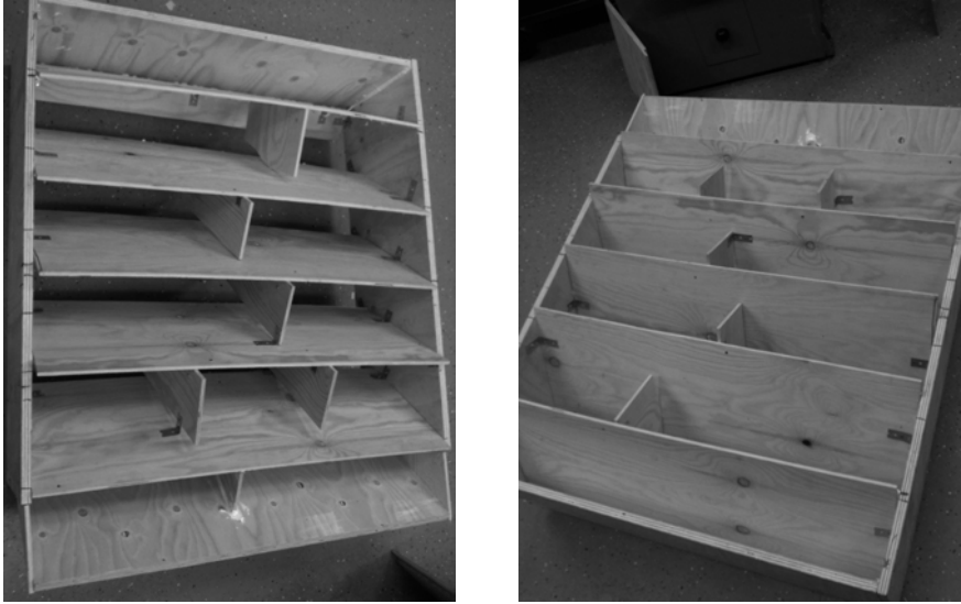
Figure 6.10.: Photos of the supporting structure of the prototype baffled panel.
