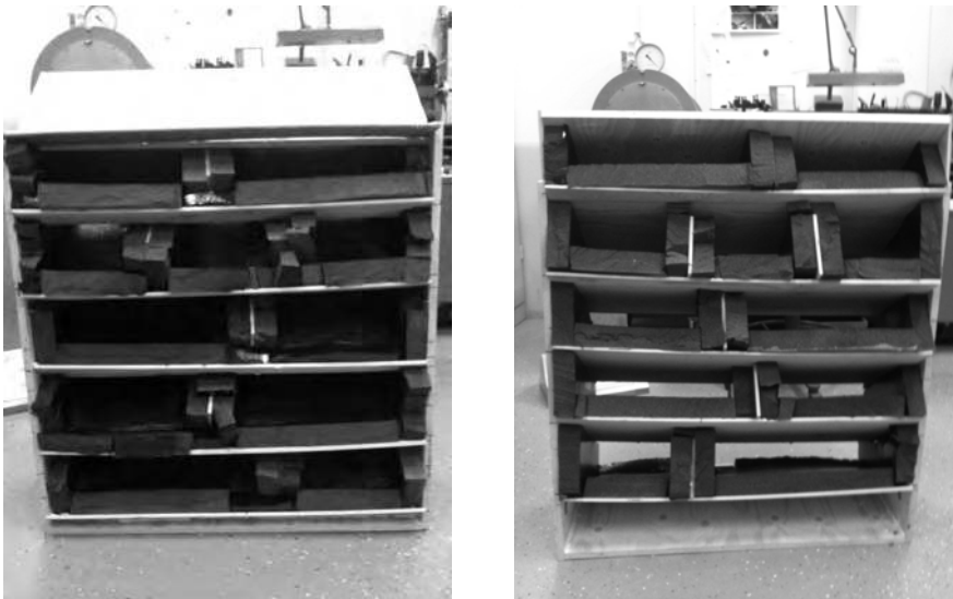
Figure 6.11.: Photos of complete prototype baffled panel from front and back.
