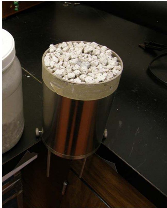
Figure 3 Pumice in impedance tube sample holder
