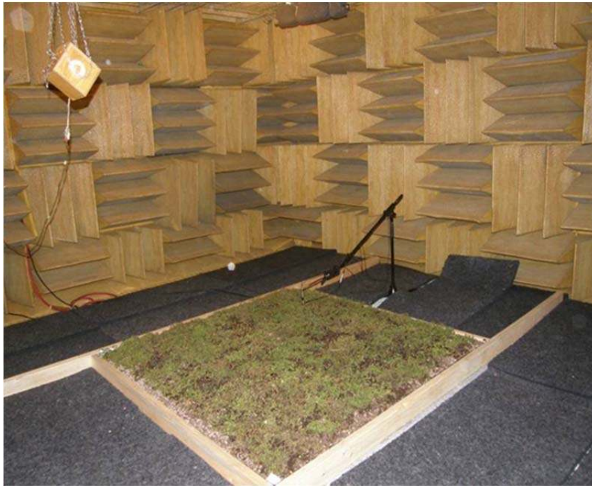
Figure 8 Set-up of vegetative vegetated roof test plot with surrounding baffles
