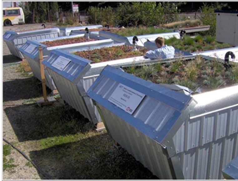
Figure 26 Roofing evaluation modules (REM)
