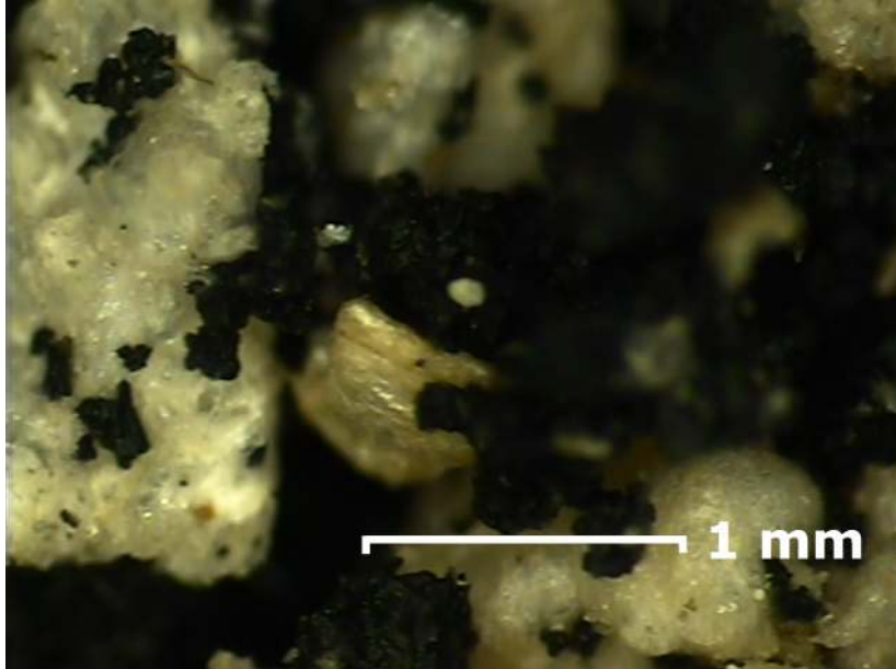
Figure 1 Microphoto of sample M-1 obtained with Mitutoyo Vision Machine. Particle of rubber, EPS and vermiculite can be observed.
