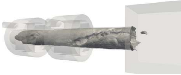
(b) Fully flashed back (FFB) flame
