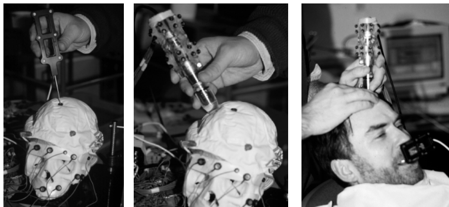
Fig. 3. Localization of markers (left) and collection of cranial surface points (middle) during the skull phantom experiment. Also, localization of skull surface points in one of the volunteer studies (right).
