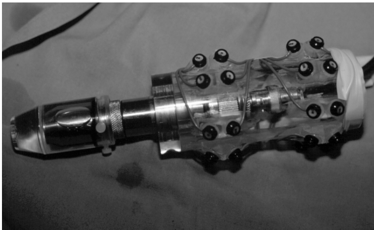
Fig. 1. Photograph showing the A-mode ultrasound transducer, the array of attached IREDS, and the offset.
