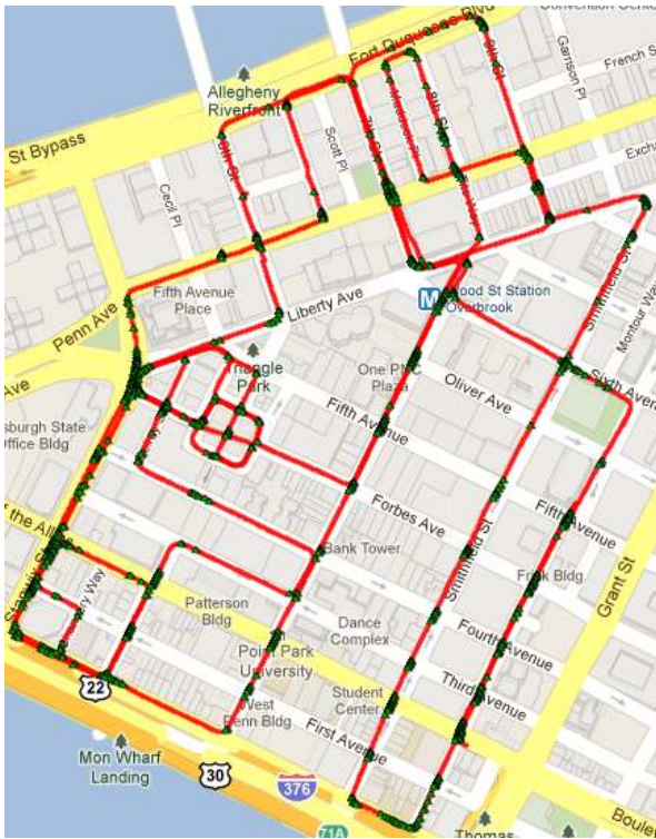
Fig. 10. Visualization of the intersection recognition experiment. Green points mark the locations classified as intersections.
