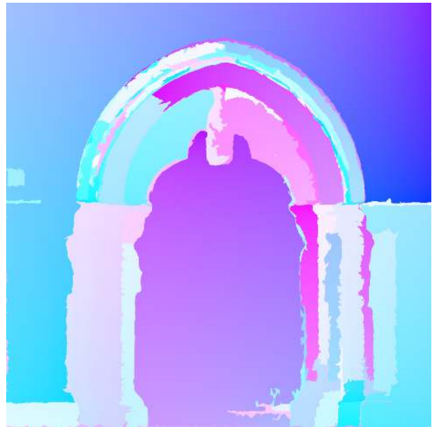
Figure 5: Colour coded UV map, to arbitrarily reassign 3D model coordinates to the 2D texture coordinates of the multiple maps.
